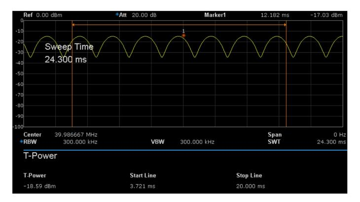
**T-Power:** The power of the signal from the start line to the stop line.
