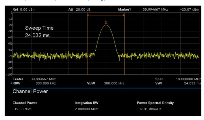
Measurement Results: Channel power and power spectral density.
